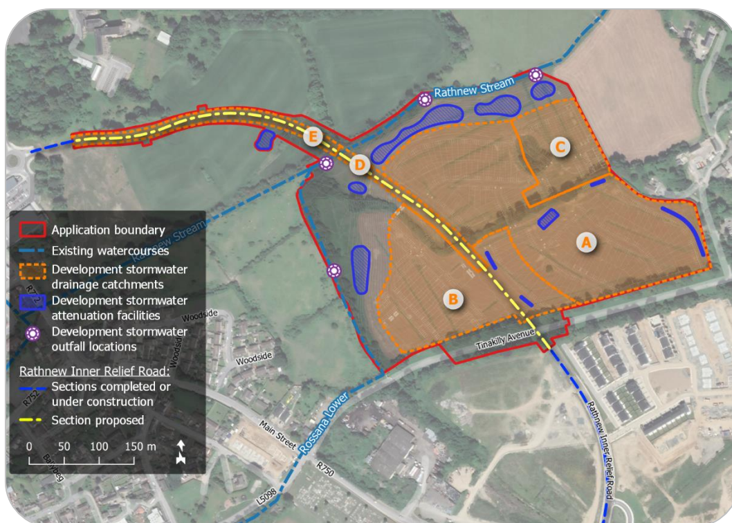
Figure 4 – Proposed final stormwater drainage arrangements (map data and imagery: EPA, OSM Contributors, Google)
